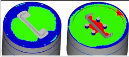
Figure 4. Results for Die A, between cap and feeder (left) and between backer and cap (right). Blue represents areas of no contact, green represents sliding surface, and red represents sticking surface.
