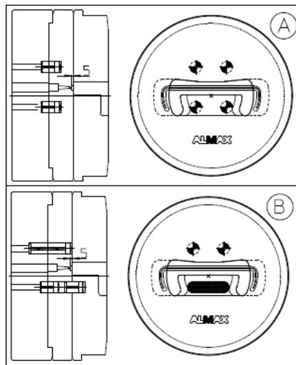
Figure 2. Schematic of the two die designs that were under investigation, showing a vertical cutaway-section (left) and a front view (right) of each die.
