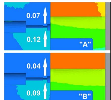
Figure 3. Deformation of the cap under load for Die A (top) and Die B (bottom) along cutaway-section (values in mm).
