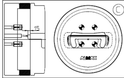
Figure 5 Schematic of Die C, showing a vertical cutaway-section (left) and a front view (right) of the die.
