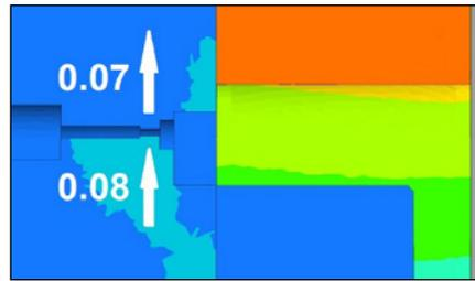
Figure 6. Deformation of the cap along cutaway section in Die C (values in mm).
