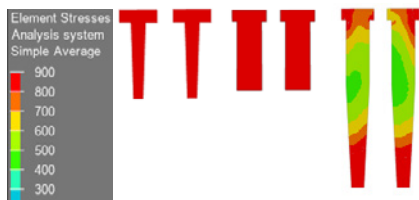
Figure 5. Numerical results in terms of Von Mises stress along the cutaway section A-A shown in Figure 2. Only the back release technology shown in the right section of Figure 4 looks acceptable; however, the bearings region is predicted to work over the plasticity limit of 850 MPa.
